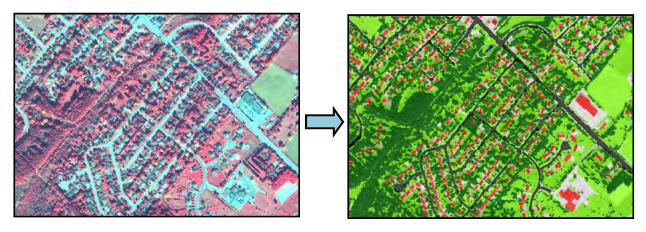
Figure 4: High resolution satellite imagery (left) used to produce digital surface cover map (right).
