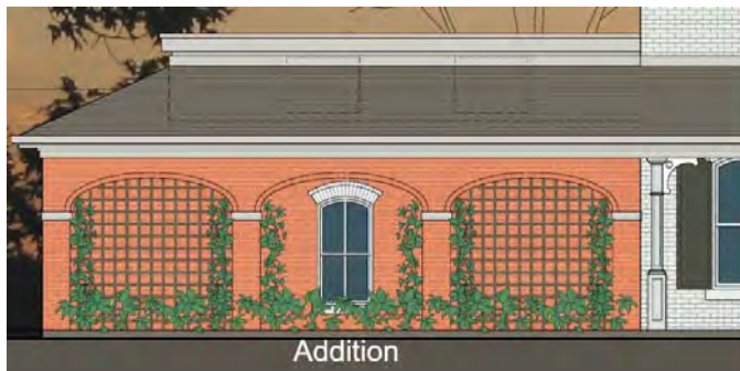
Trellis Frames Inset into Masonry Wall Panels- Dashed Lines Indicate Concealed Rooftop Mechanical Units
