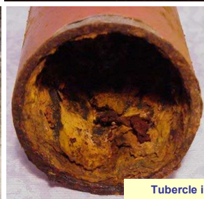
Watermain- Pitting corrosion
