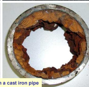
Watermain- Pitting corrosion
