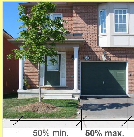
Typical townhouse with front garage limited to 50% or less of total unit width
