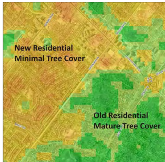
Thermal imagery illustrating the contrast in temperatures observed between neighbourhoods with varying tree cover. Image courtesy of Natural Resources Canada.
