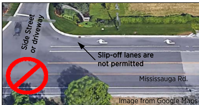
Figure 2.5: Increases to the street pavement width as a result of development is not permitted.
