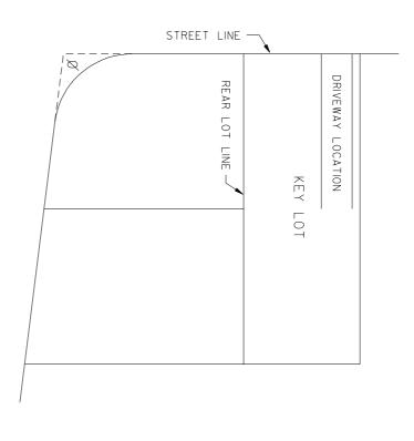
I. DRIVEWAY LOCATIONS AS PER THIS STANDARD ARE VALID WHEN THE ANGLE Ø IS EQUAL TO OR LESS THAN 115°
