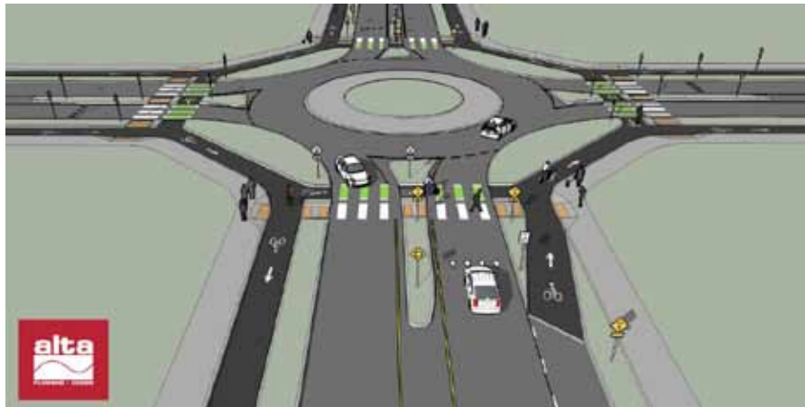
Figure V-5: Protected bike lane (or separated cycle track) at a roundabout with dedicated bicycle crossings Bicycle Bypass (Image credit: Alta Planning)
