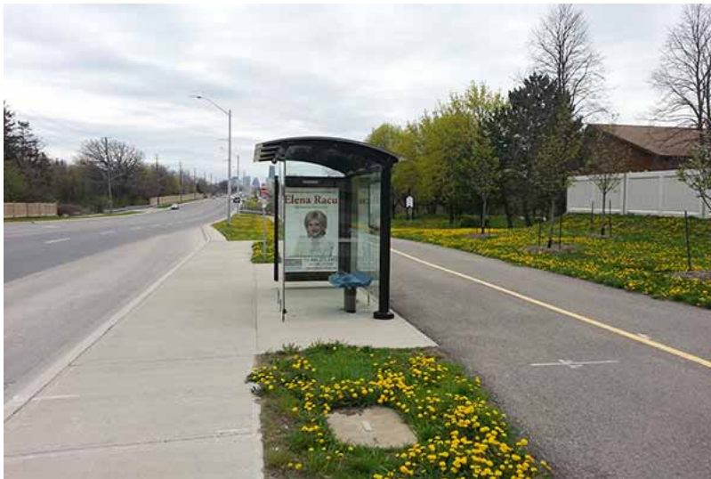
Figure V-26: Bus stop with separate loading platform, in Mississauga, on Burnhamthorpe Road East. This design keeps the trail behind the stop, and minimizes pedestrian-cyclist conflicts.
