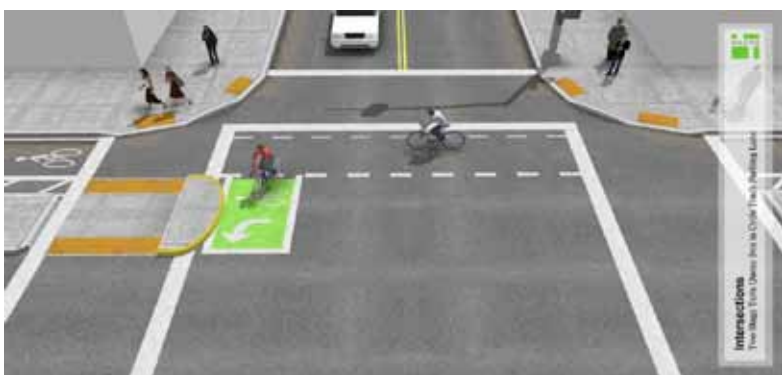
Figure V-12: Two-stage turn queue boxes are placed in a protected area such as in front of an on-street parking lane or between a bicycle lane and the pedestrian crossing. (Image credit: NACTO Urban Bikeway Design Guide )
