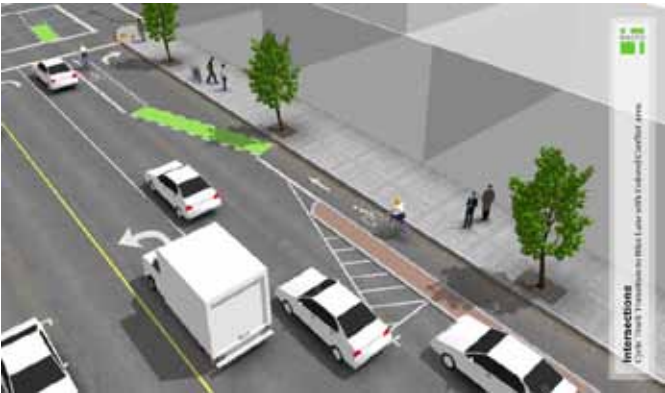
Figure V-3: A mixing zone is where a separated bicycle lane transitions to a conventional bike lane. (Image credit: NACTO Bikeway Design Guide , 2012)
