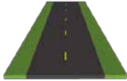
Yellow Broken Centreline
