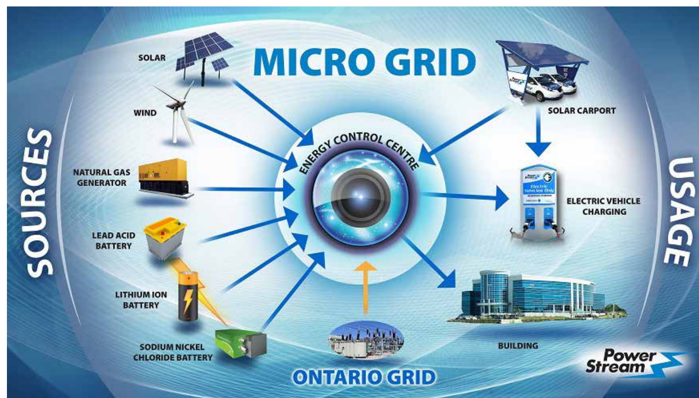
Figure 4.1 - A grid-connected microgrid network
