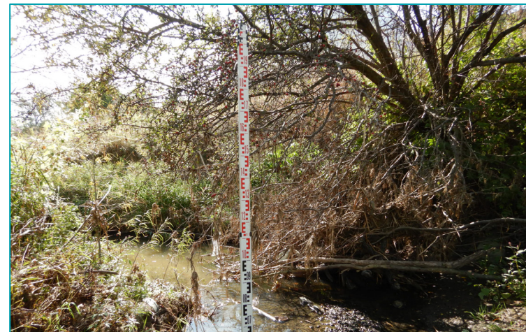
1 - Bank and slope erosion scar with vertical exposure and vegetation failure into the channel.
