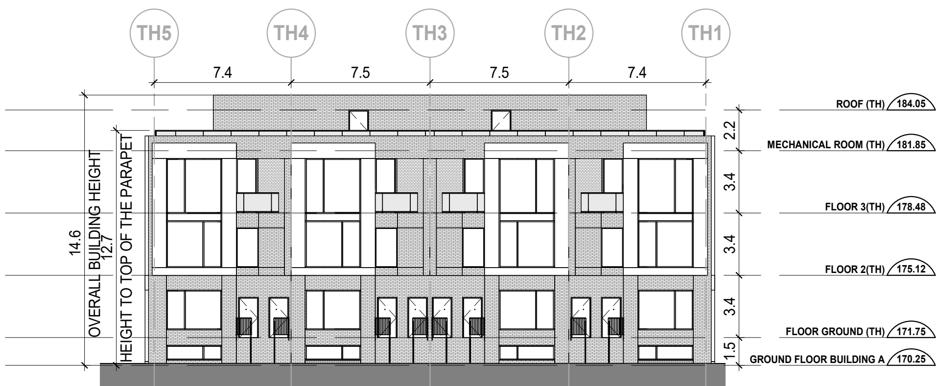
2 Block 2 & 3 Typical Townhouse - West Elevation SCALE: 1 : 200
