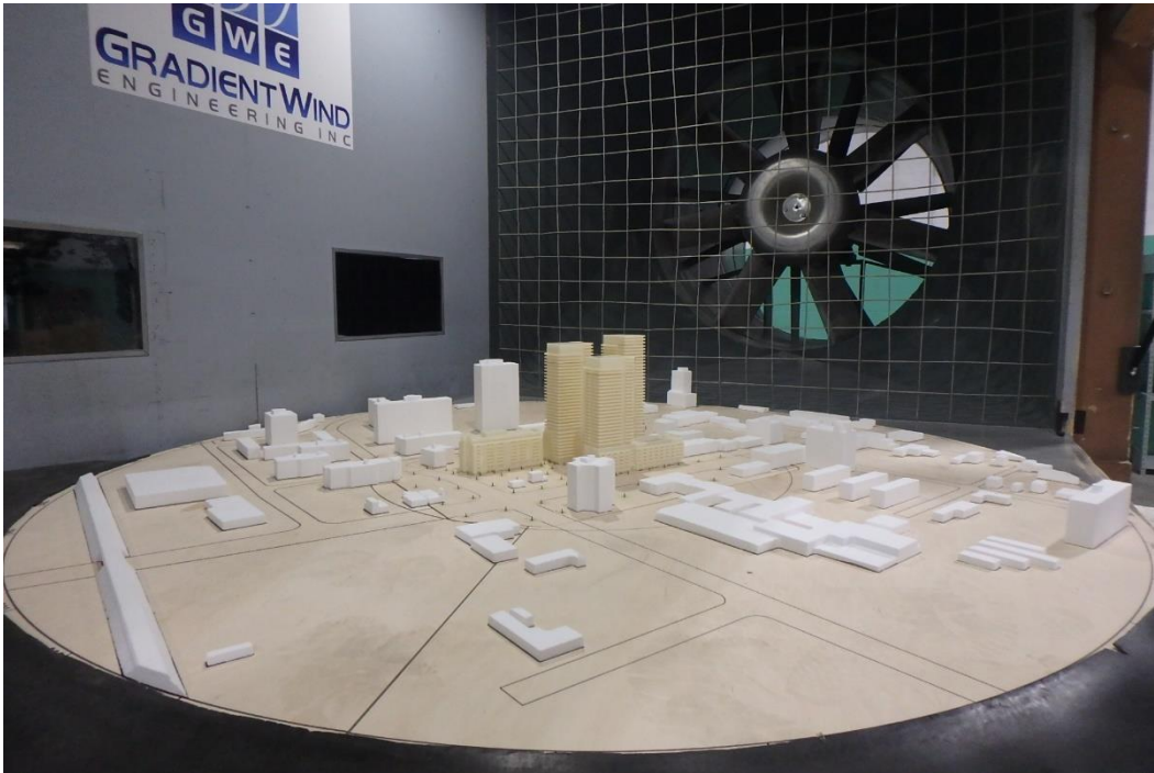
PHOTOGRAPH 3: STUDY MODEL INSIDE THE GWE WIND TUNNEL LOOKING DOWNWIND
