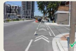
Pavement markings through intersections
