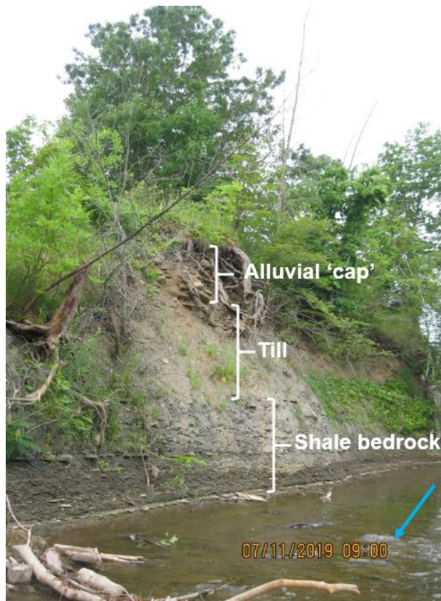
Photo 7. Generalized stratigraphy of the terrace scarp within the 2935 Mississauga Road property.
