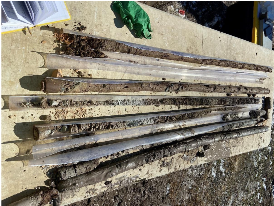
Photo 14: Soil cores extracted from borehole BH8 to a depth of 7.6 m with Geoprobe continuous core sampling method using Macrocore MC5 dual tube sampling system.
