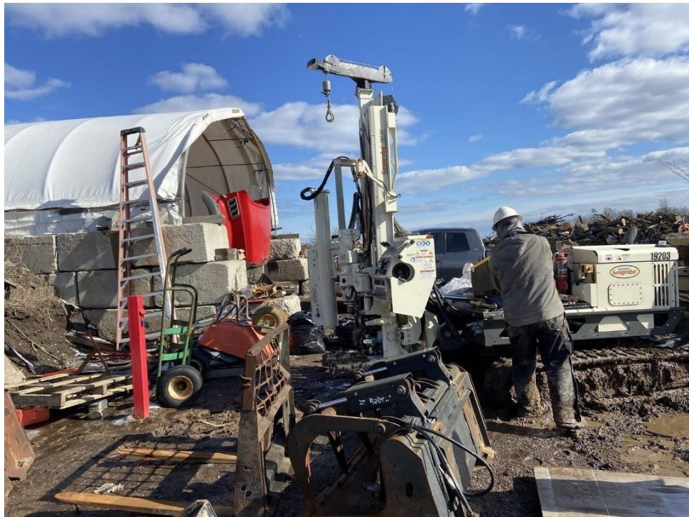
Photo 10: Geoprobe drilling borehole BH6-B beside monitoring well MW6-21 near former tanks.
