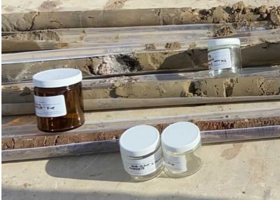
Photo 11: Soil cores extracted from borehole BH6-B to a depth of 6.1 m with Geoprobe continuous core method using Macrocore MC5 dual tube sampling system.
