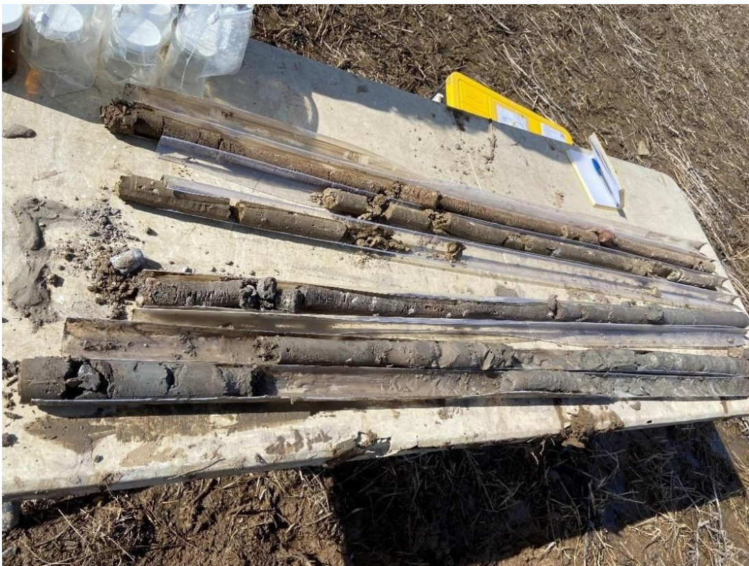
Photo 4: Soil cores extracted from borehole BH1-B to a depth of 6.1 m with Geoprobe continuous core sampling method using Macrocore MC5 dual tube sampling system.
