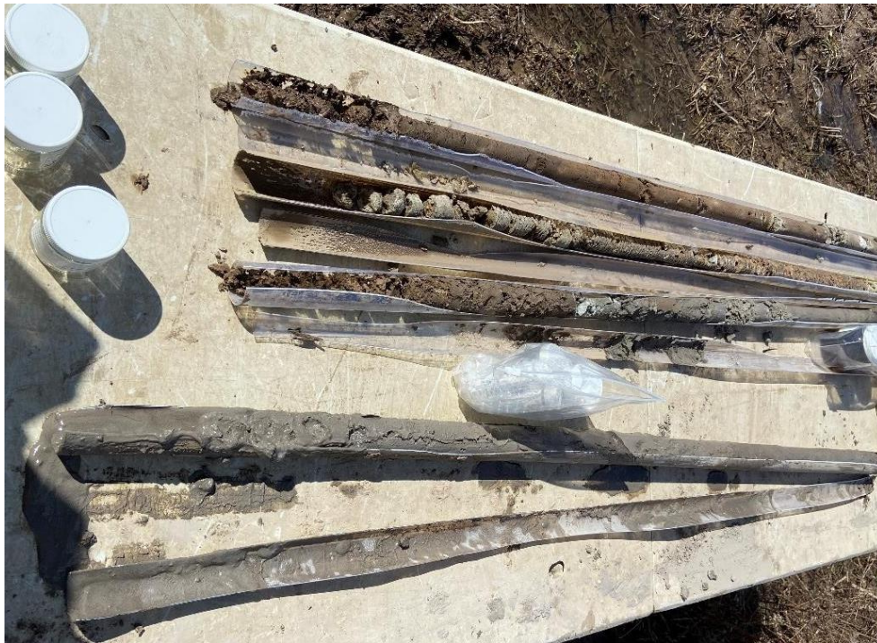
Photo 8: Soil cores extracted from borehole BH5-B to a depth of 6.1 m with Geoprobe continuous core sampling method using Macrocore MC5 dual tube sampling system.
