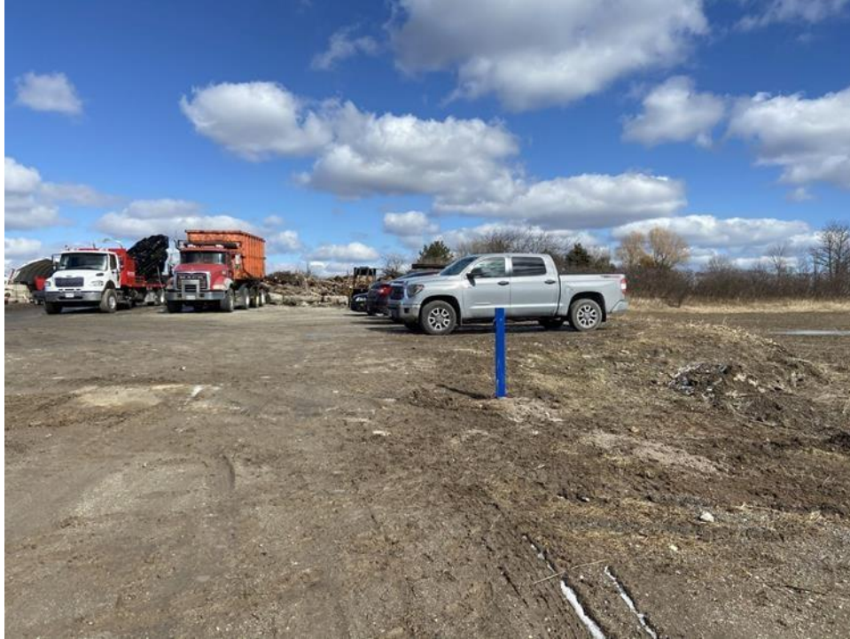
Photo 13: Groundwater monitoring well MW8-22 installed at BH8 at edge of driveway.
