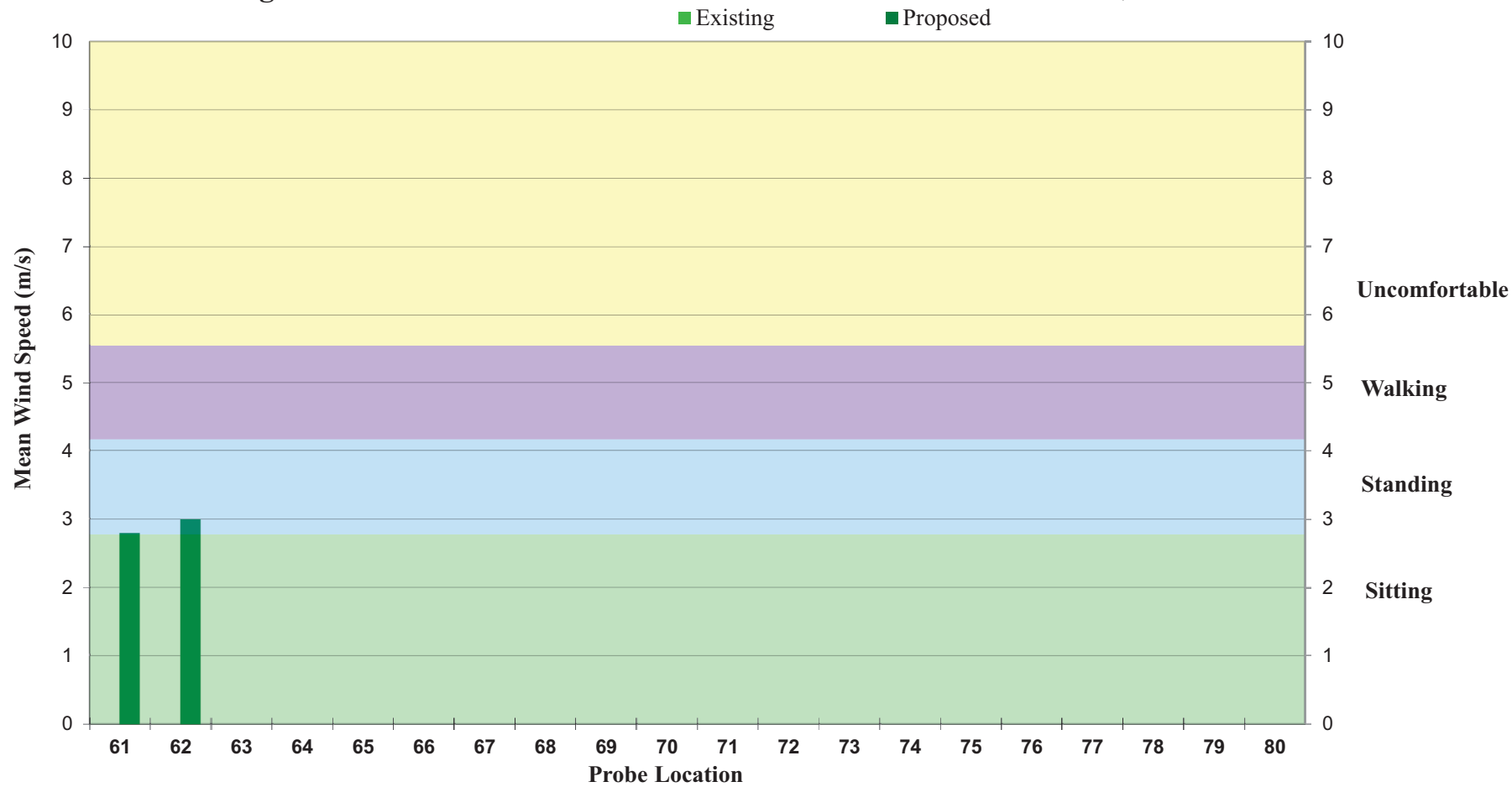
Figure 6a: WINTER - Wind Speed Exceeded 20% of the Time (Locations 61 to 62).
