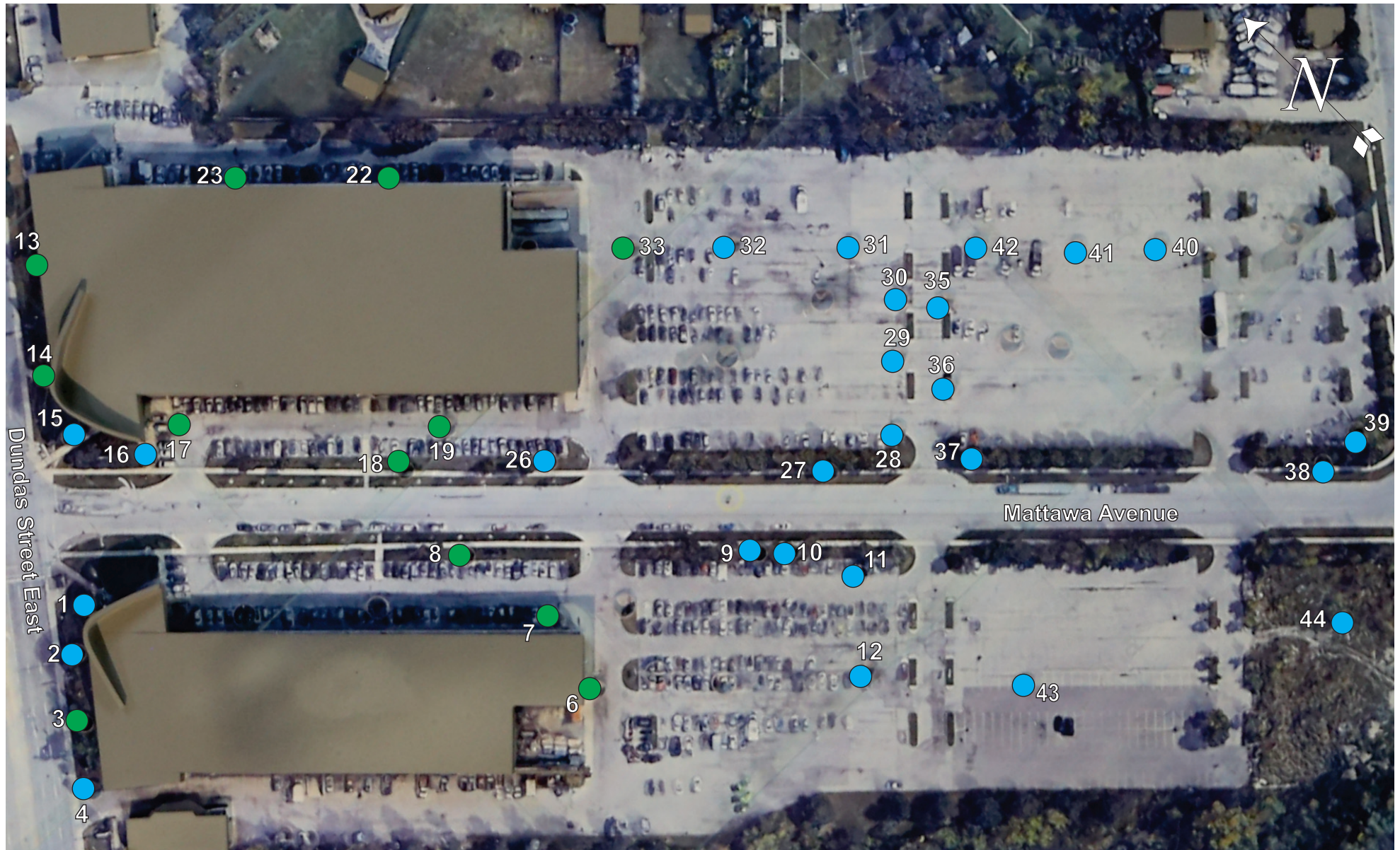
Figure 7c: Pedestrian level wind velocity comfort categories.
