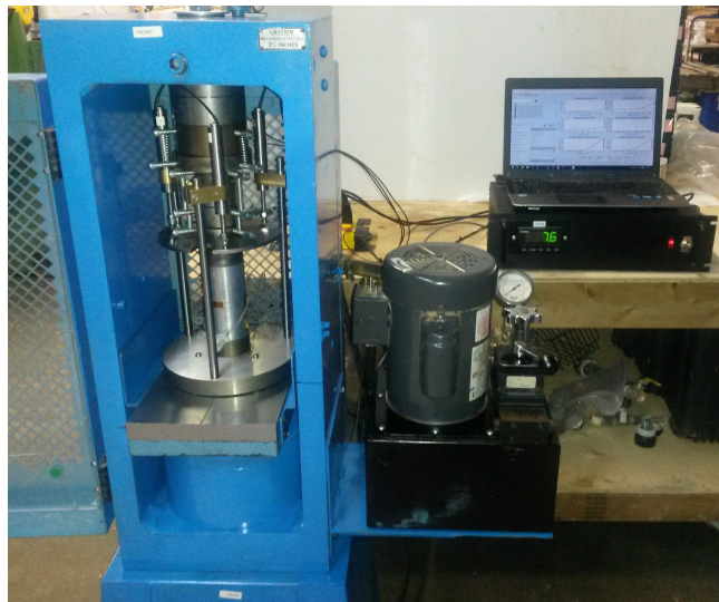
Figure 1: Forney loading frame setup for UCS testing.
