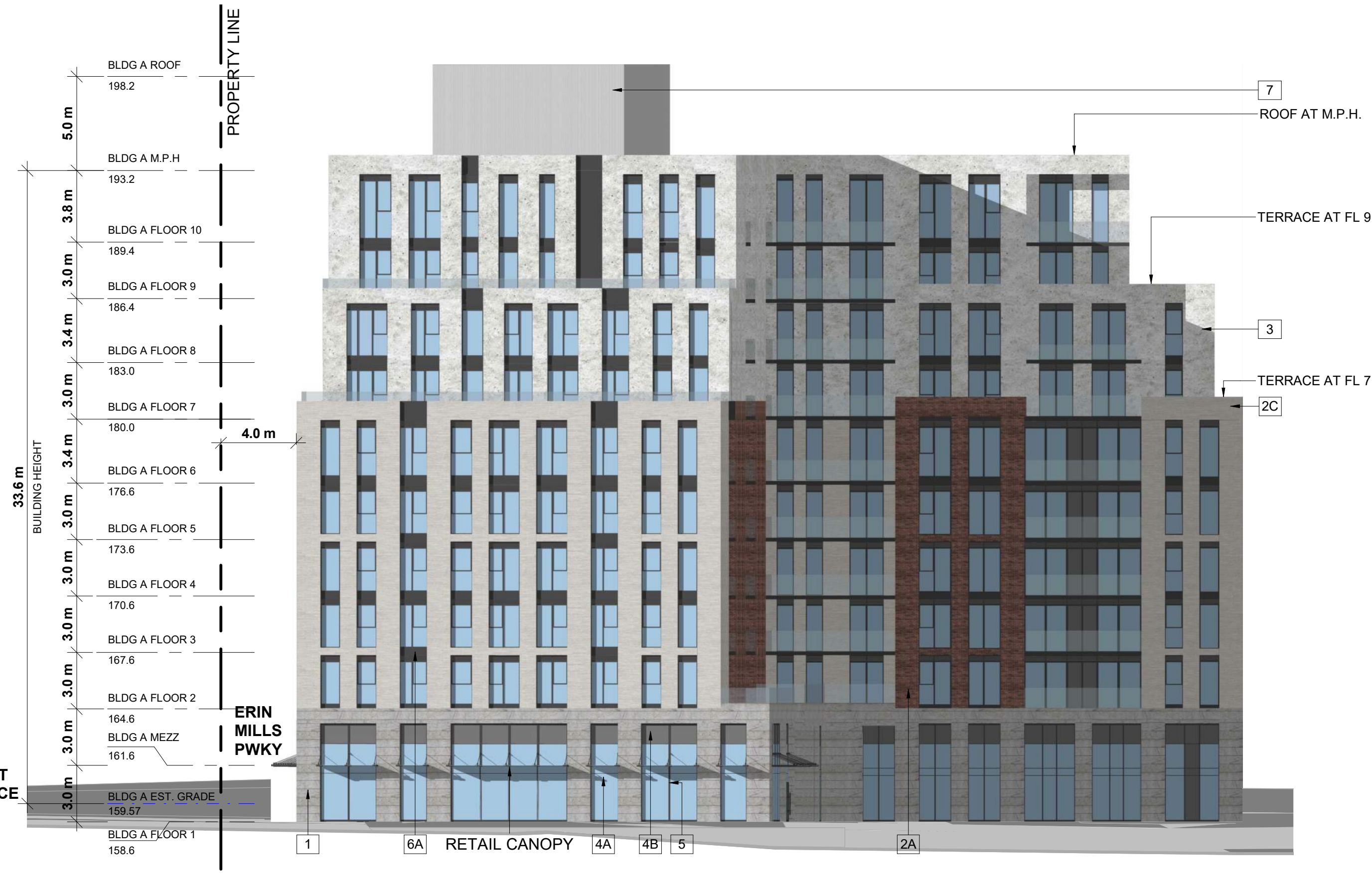
1 BLDG A SOUTH ELEVATION SPA310 1:200
