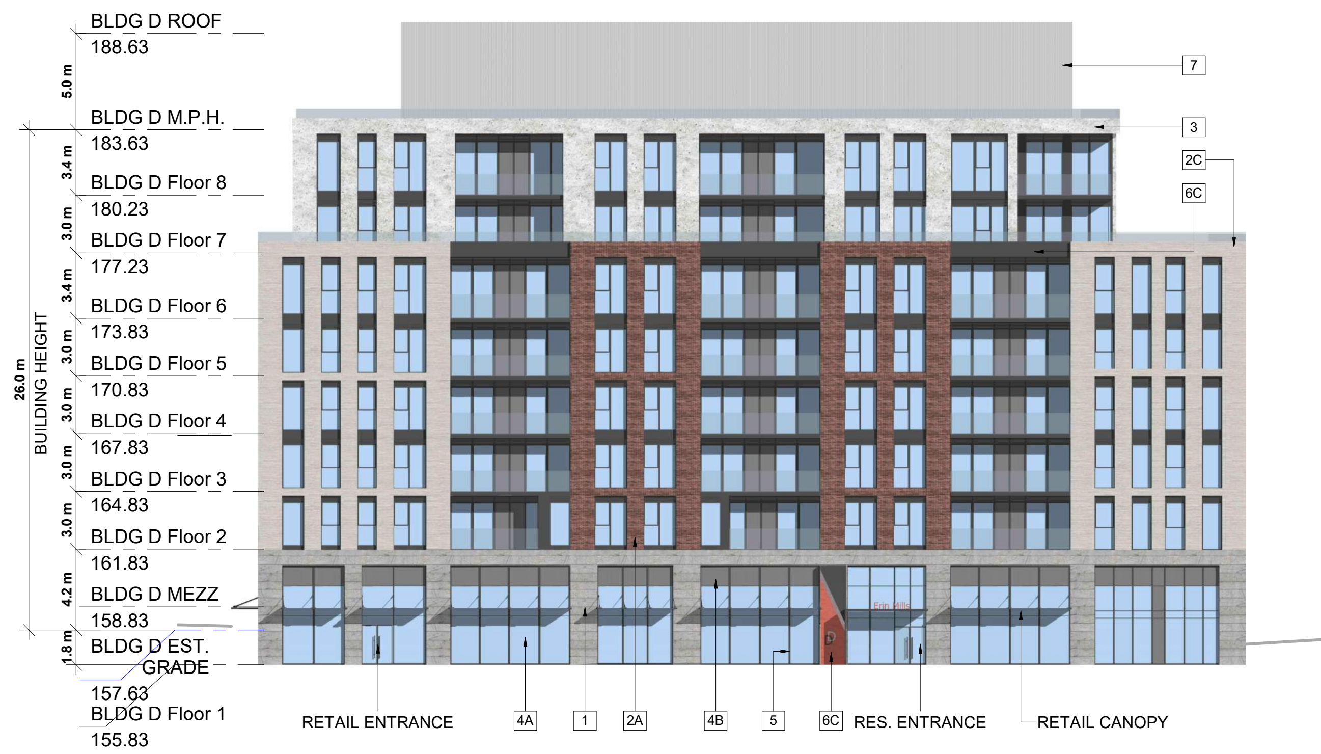
3 BLDG D WEST ELEVATION SPA314 1:200
