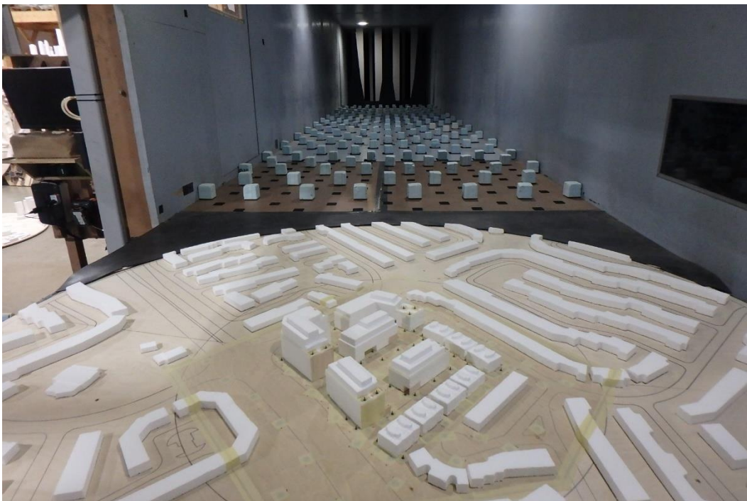
PHOTOGRAPH 4: STUDY MODEL INSIDE THE GWE WIND TUNNEL LOOKING UPWIND
