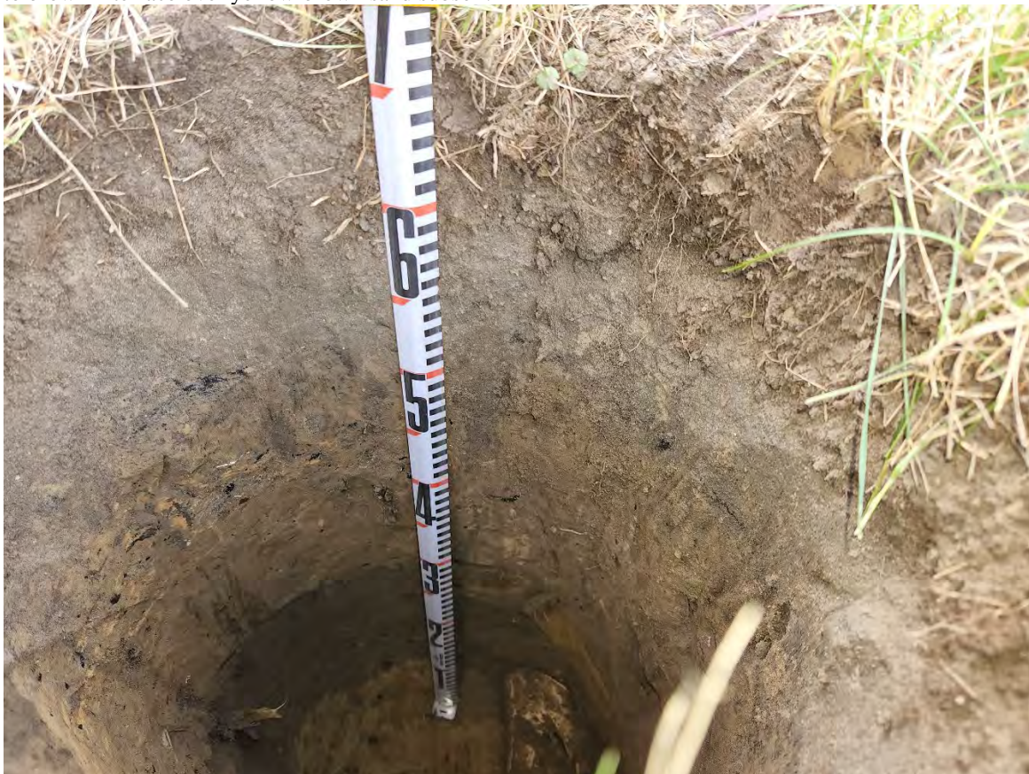
Image 6: Deep disturbed test pit with yellow clay drainage tile at bottom.
