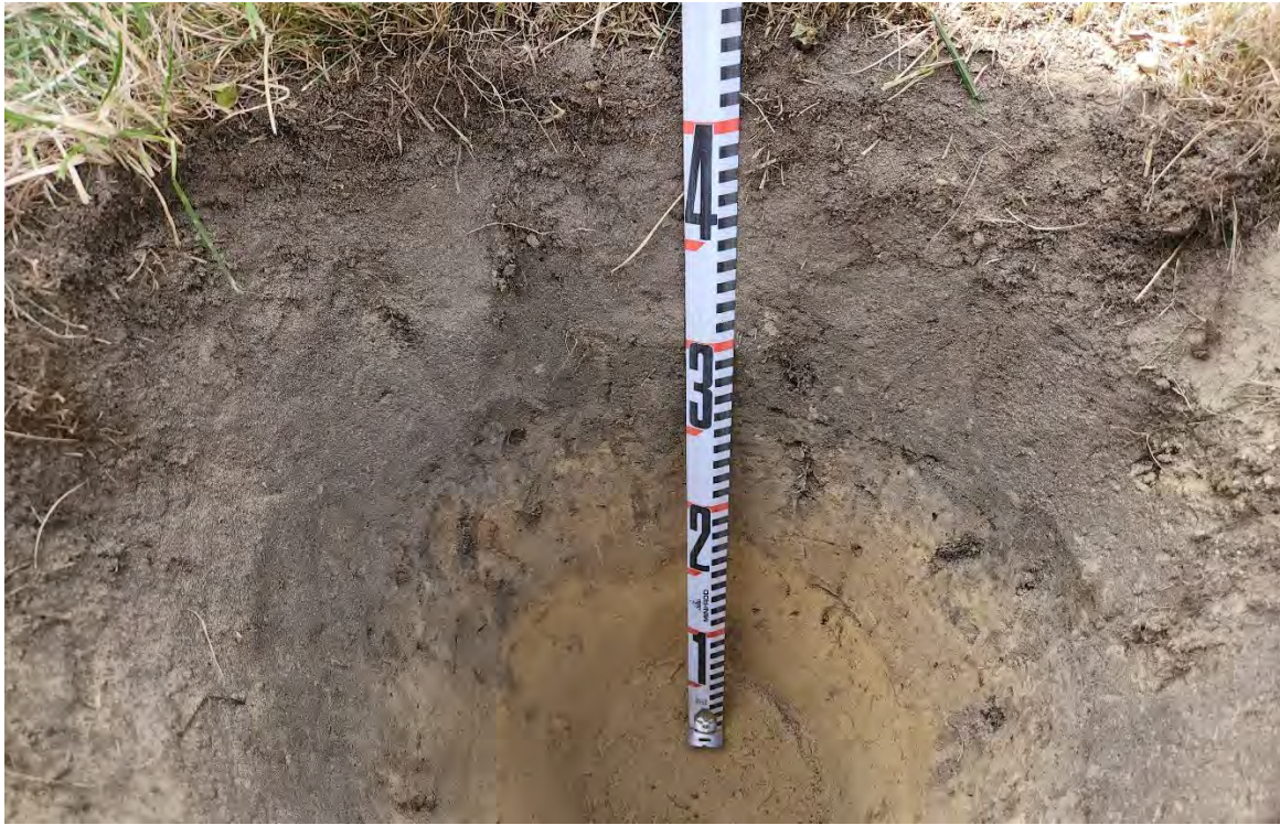
Image 5: Disturbed test pit profile in former lawn bowling green with brown silty sand over mottled yellow-brown to brown interface over yellow-brown sand subsoil.
