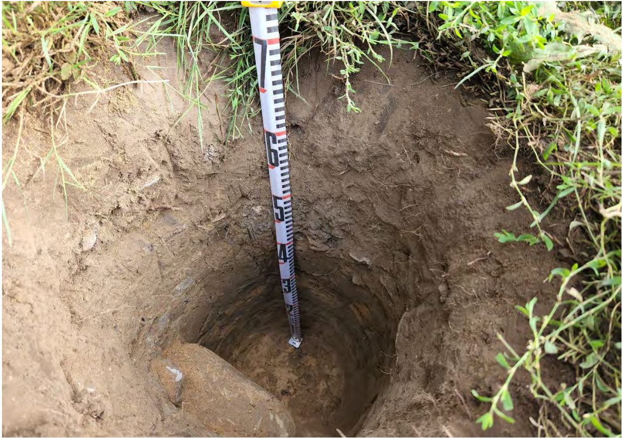
Image 13: Deep disturbed test pit along the west side of the 84 High Street house.
