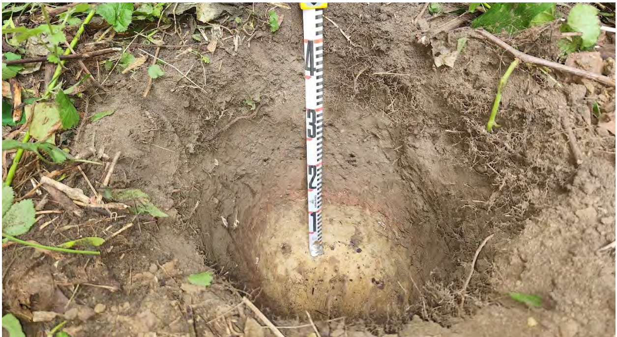
Image 4: Disturbed test pit with light brown silty sand over a red clay lens over yellow sand subsoil.
