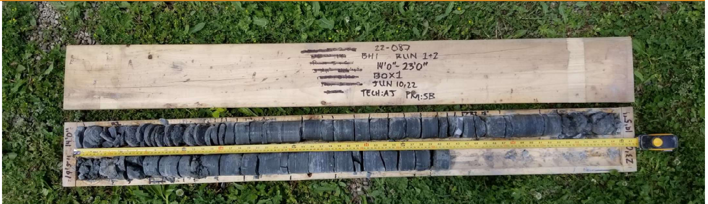
Run 1 - Depth: 4.3 to 5.5 m below grade (Elev. 133.6 to 132.4 m) Run 2 - Depth: 5.5 to 7.0 m below grade (Elev. 132.4 to 130.9 m)
