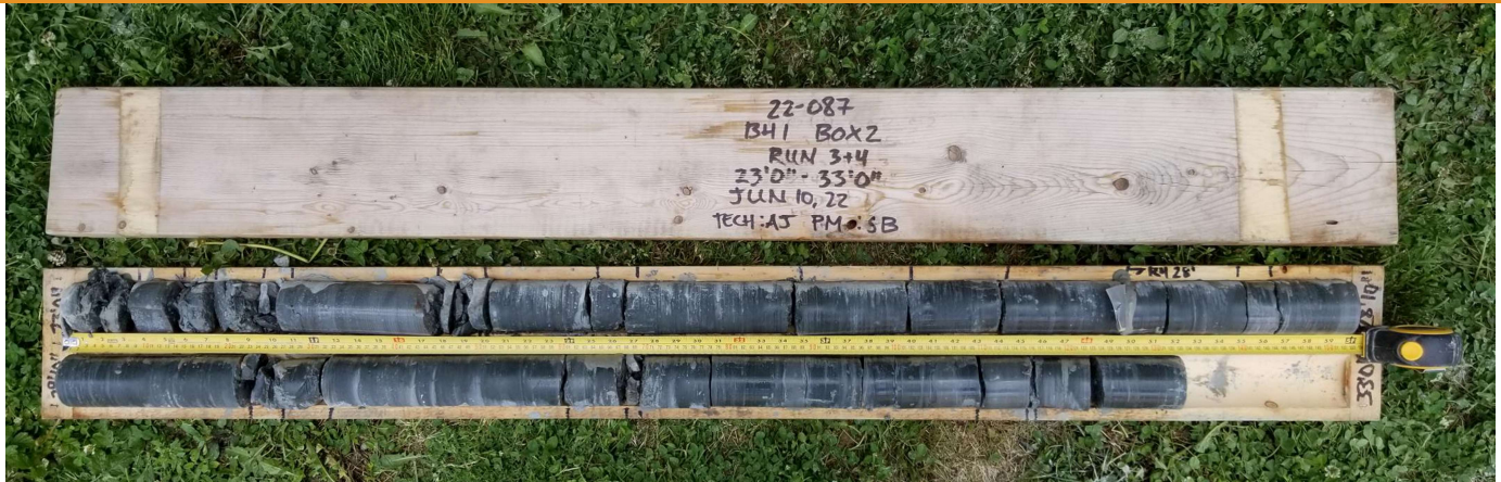
Run 3 - Depth: 7.0 to 8.5 m below grade (Elev. 130.9 to 129.4 m) Run 4 - Depth: 8.5 to 10.1 m below grade (Elev. 129.4 to 127.8 m)
