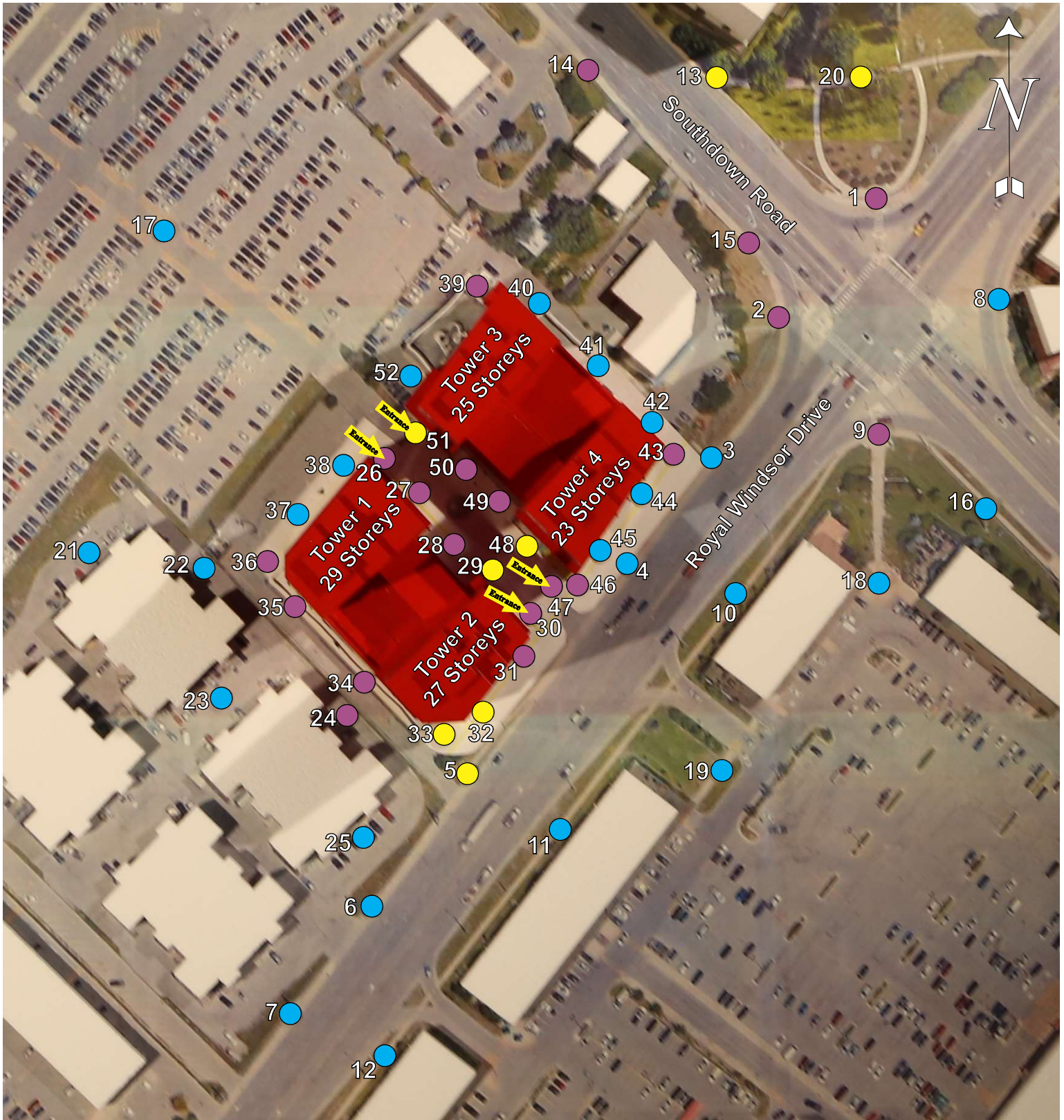
Figure 7b: Pedestrian level wind velocity comfort categories.
