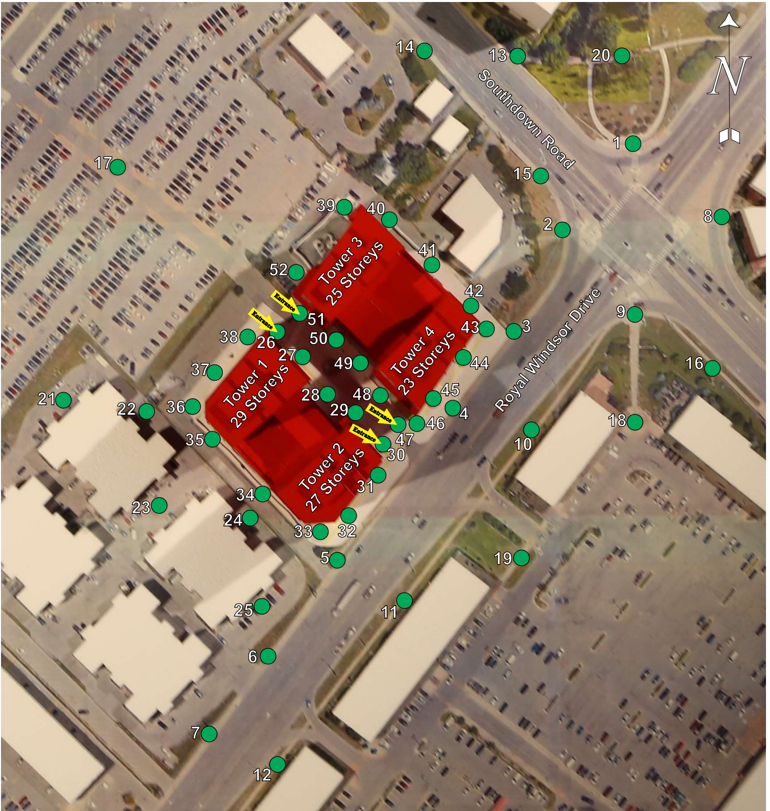
Figure 4: Location plan for pedestrian level wind velocity measurements. 25
