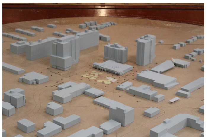
Image 2A: Wind Tunnel Study Model – Existing Configuration (Tested in February 2022)
