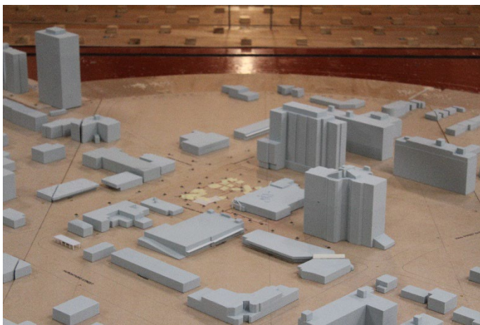
Image 2A: Wind Tunnel Study Model – Existing Configuration (Tested in February 2022)
