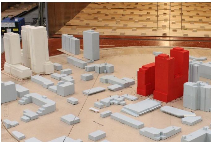
Image 2D: Wind Tunnel Study Model – Future Configuration (Tested in December 2022)
