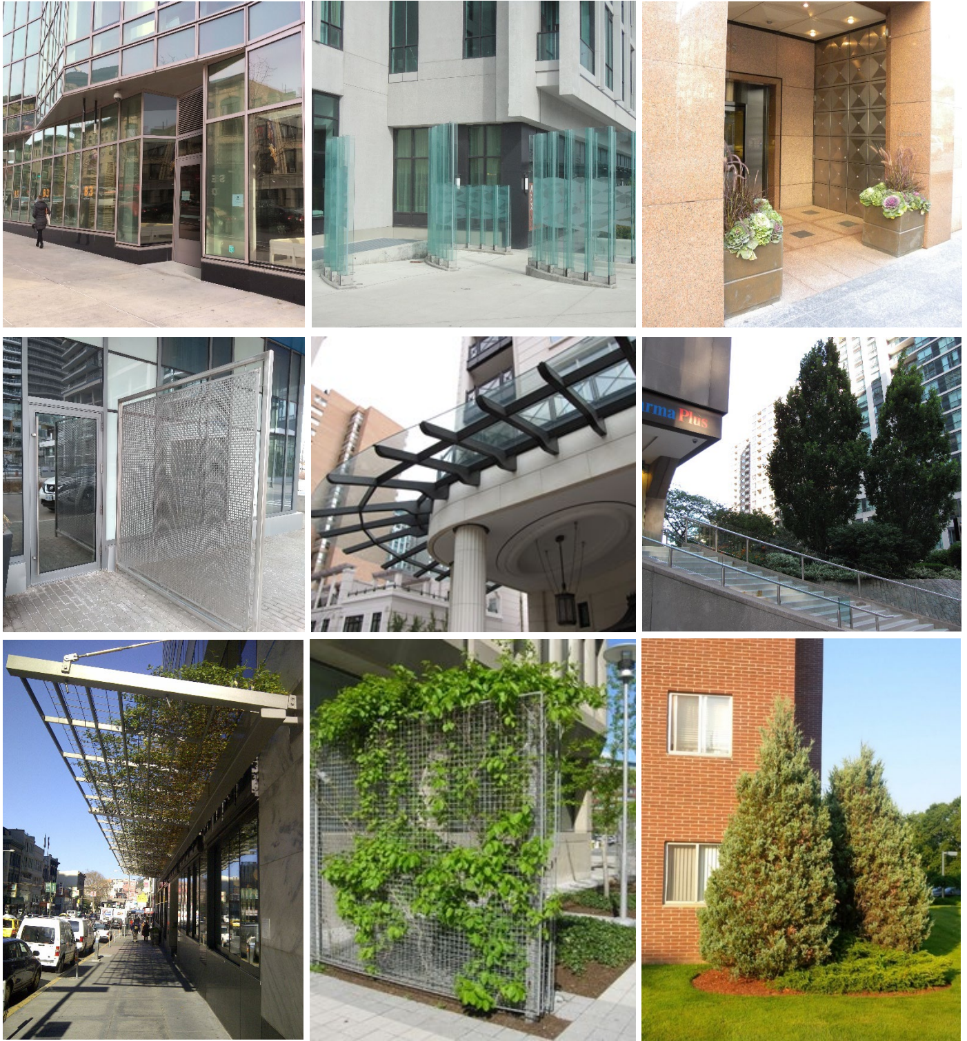
Image 7: Examples of Wind Control Options Applicable for Grade Level
