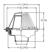
ENGINEERING SPECIFICATION: ZURN Z-105 "Control-Flo" roof drain for dead -level or sloped roof construction, Dura-Coated cast iron body. "Control-Flo" weir shall be linear functioning with integral membrane flashing clamp/ gravel guard and Poly-Dome. All data shall be verified proportional to flow rates.
