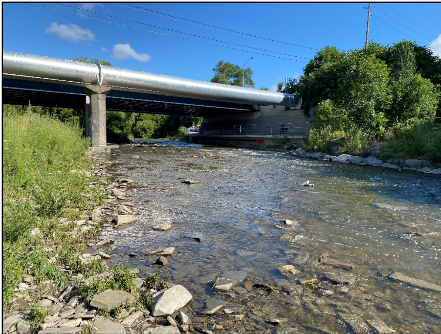
9. Etobicoke Creek – Reach ET2 – Downstream of Lakeshore Rd – View of main channel downstream of Lakeshore Rd bridge. Main channel passes through the eastern bridge opening. Wide, shallow channel with platey substrate derived from local shale bedrock.
