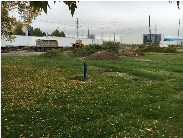
5. View of the fill piles at the central-western portion of the Site, looking southwest. Note the existing monitoring well (BH4) in this area.
