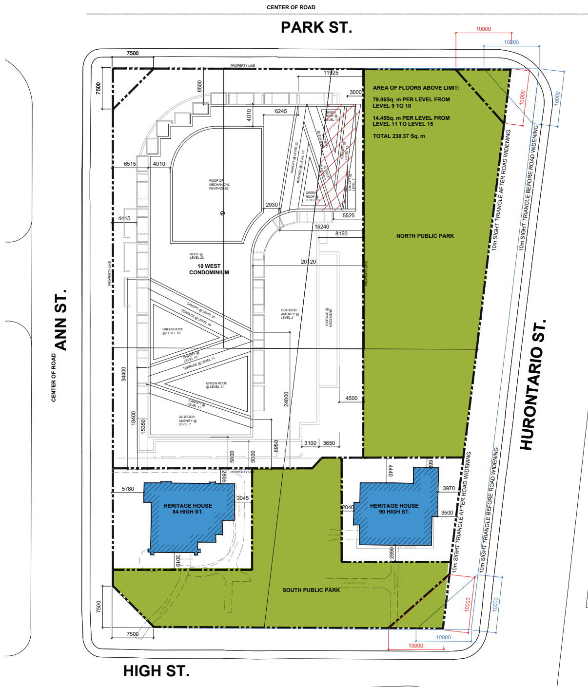
Proposed Site Plan, with the retained heritage buildings in blue and proposed public park space in green (CORE Architects, 2022, annotated by ERA).
