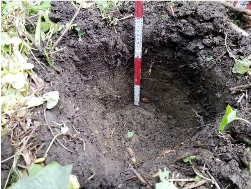
Image 5: Test pit profile showing natural stratigraphy with gleysolic profile.
