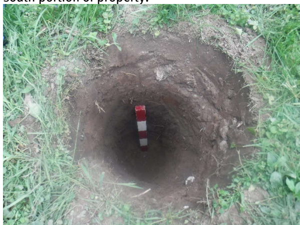
Plate 10: Typical test pit within the northwest portion of the property with buried topsoil under layers of fill.
