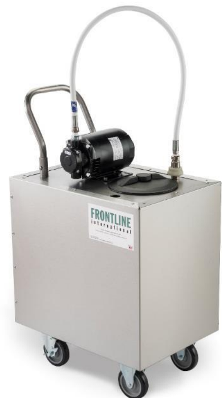
Figure 4: Mobile tank system with pump. Dimensions of the 74-gallon model are 35" L x 26" W x 39" H (889 mm x 660 mm x 978 mm). Smaller 47-gallon versions of this container are also available. Other manufacturers may have similar models in different sizes.
