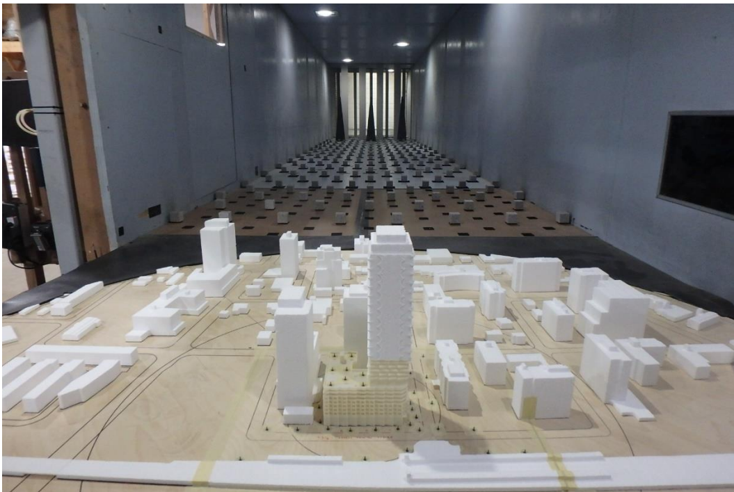
PHOTOGRAPH 4: PROPOSED STUDY MODEL INSIDE THE GWE WIND TUNNEL LOOKING UPWIND
