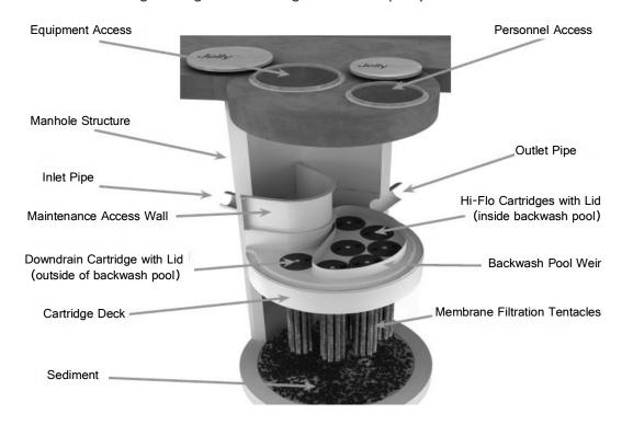
Figure I. Cut-away graphic of a Jellyfish® Filter manhole with 6 hi-flo cartridges and I draindown cartridge
