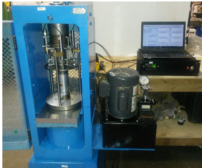
Figure 1: Forney loading frame setup for UCS testing.
