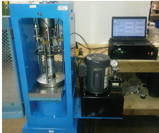
Figure 1: Forney loading frame setup for UCS testing.
