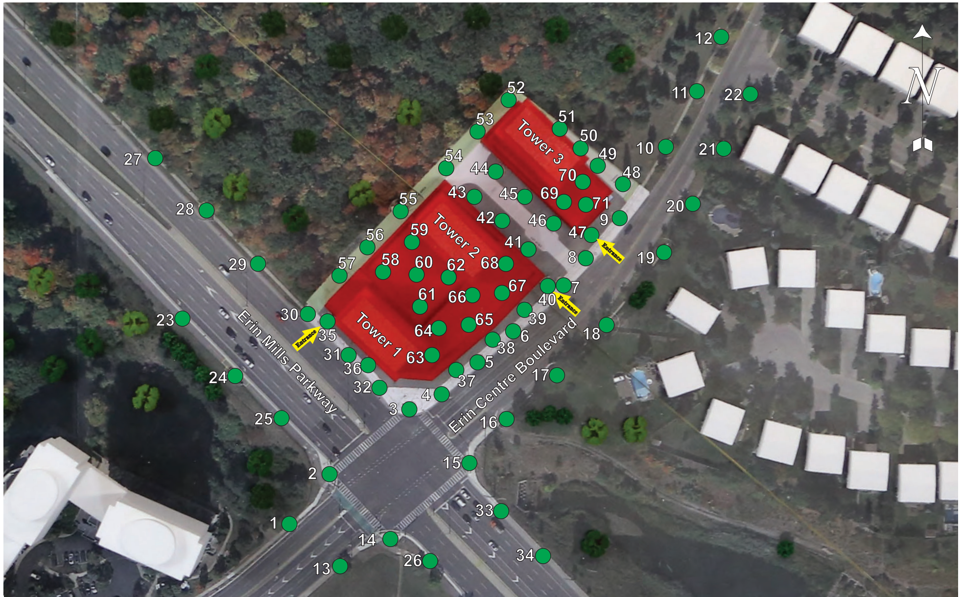
Figure 4: Location plan for pedestrian level wind velocity measurements.
