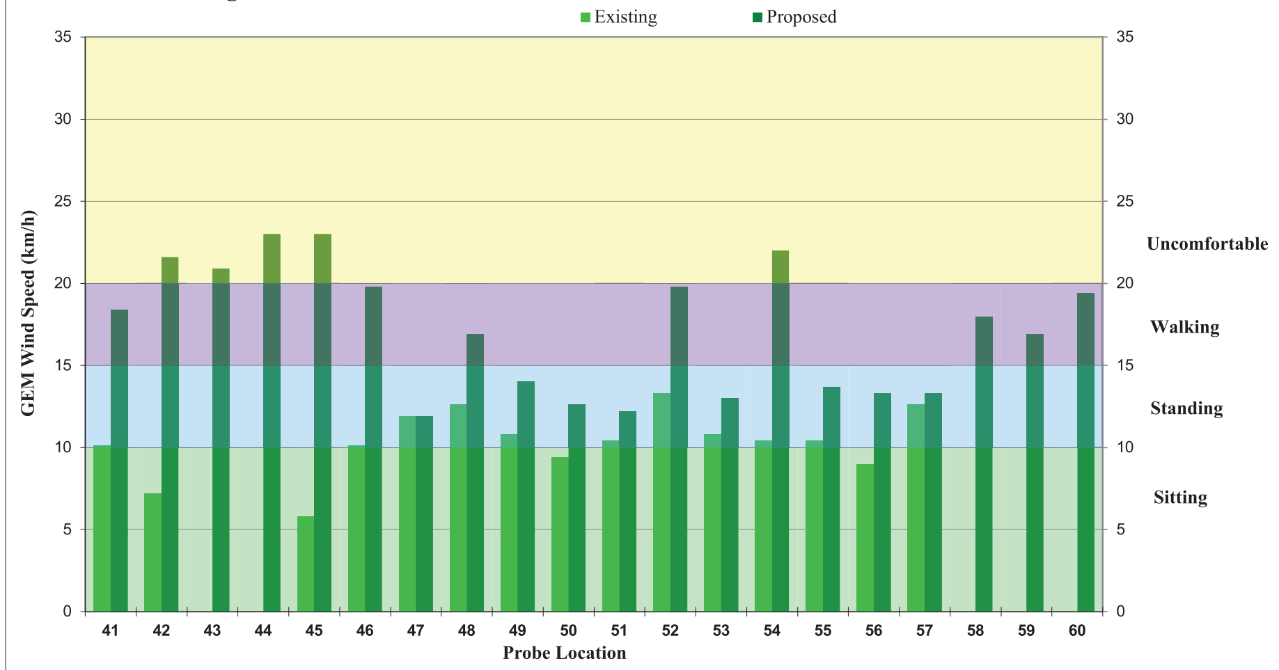
Figure 6a: WINTER - GEM Wind Speed Exceeded 20% of the Time (Locations 41 to 60).
