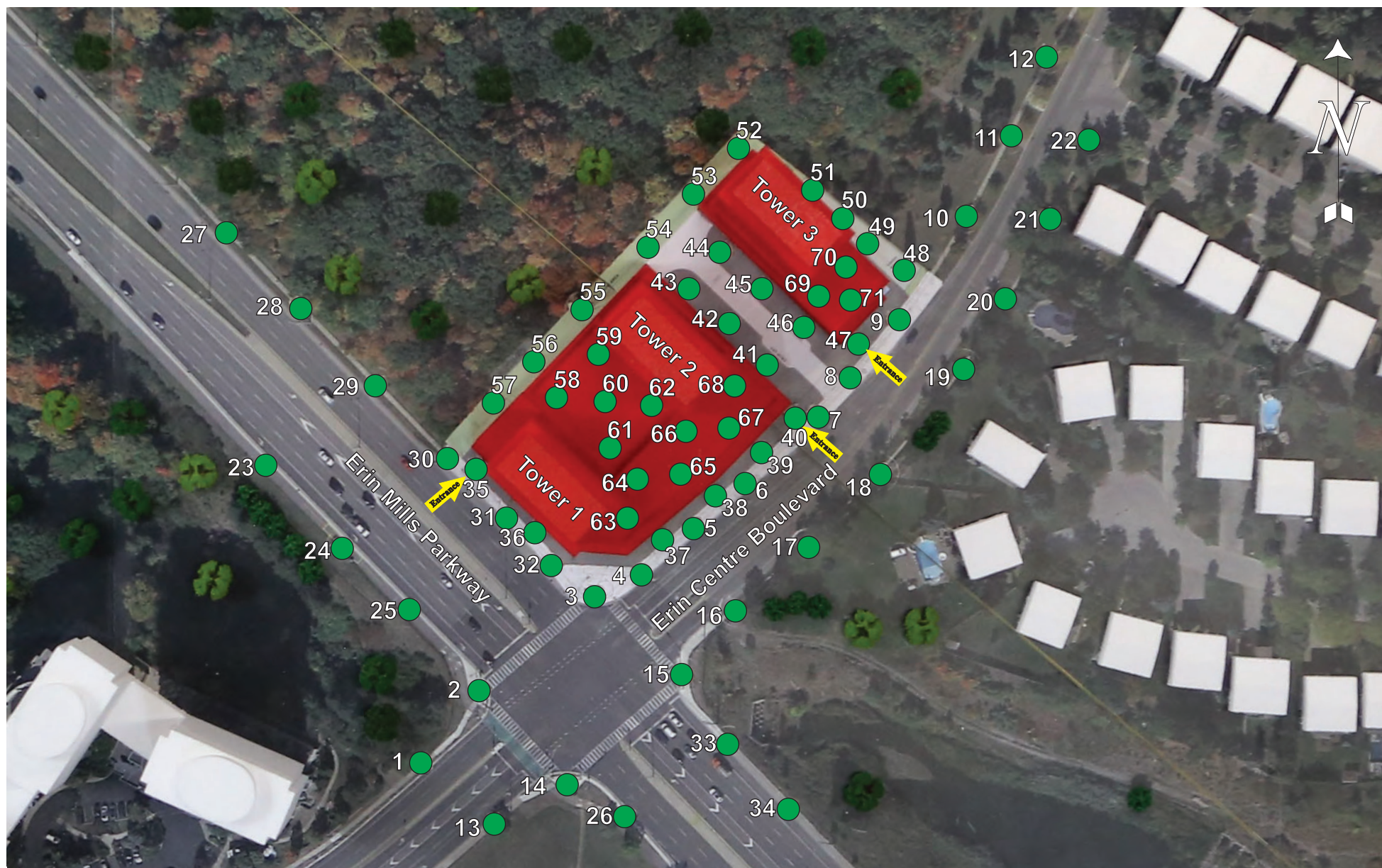
Figure 9b: Pedestrian level wind velocity safety criteria.
