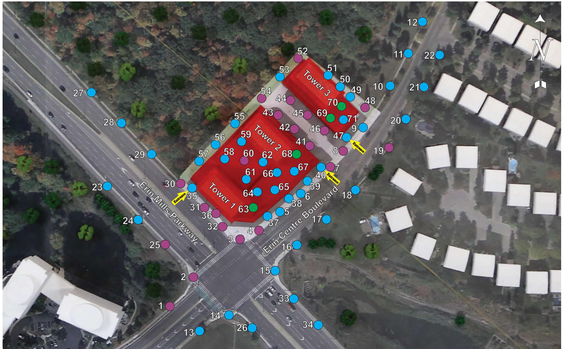
Figure 7d: Pedestrian level wind velocity comfort categories.
