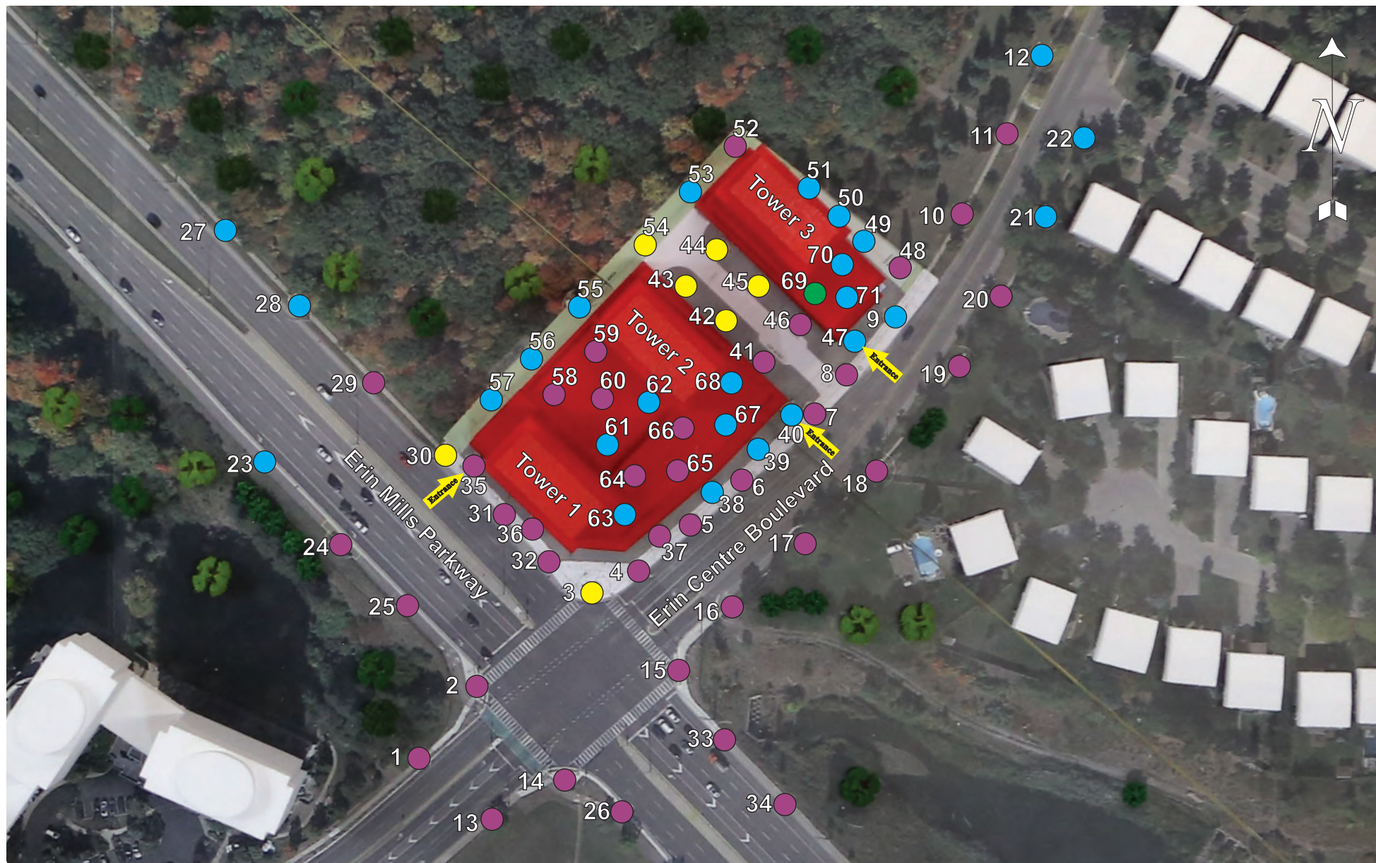
Figure 7b: Pedestrian level wind velocity comfort categories.
