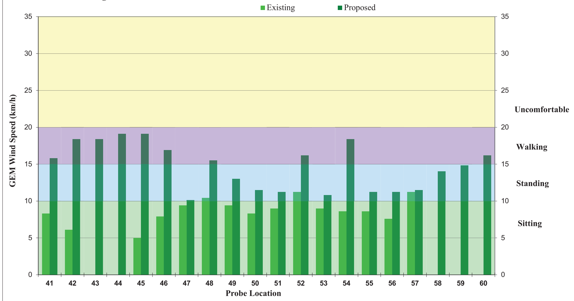
Figure 6b: SUMMER - GEM Wind Speed Exceeded 20% of the Time (Locations 41 to 60).
