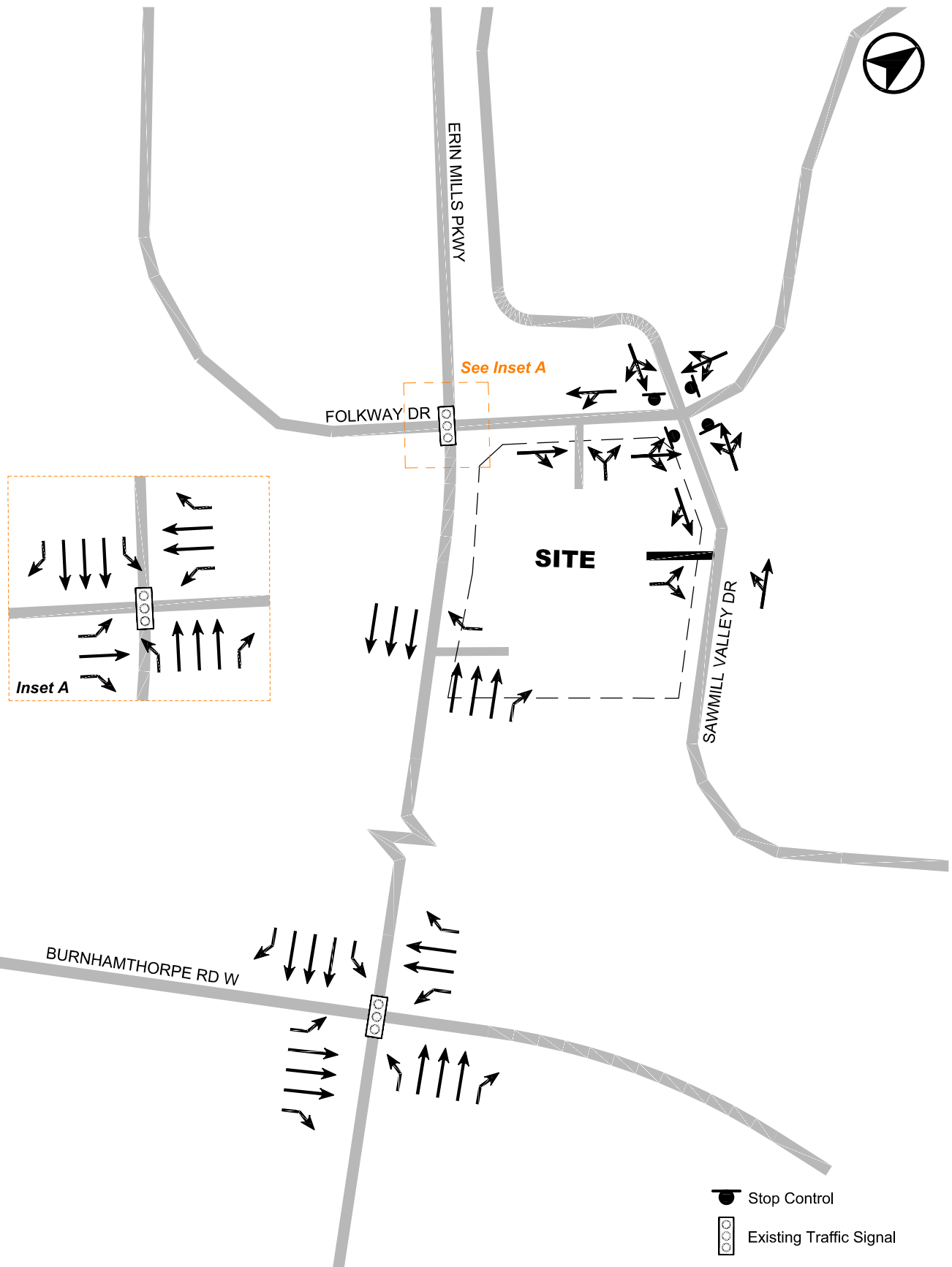
FIGURE 6 FUTURE LANE CONFIGURATION AND TRAFFIC CONTROL
