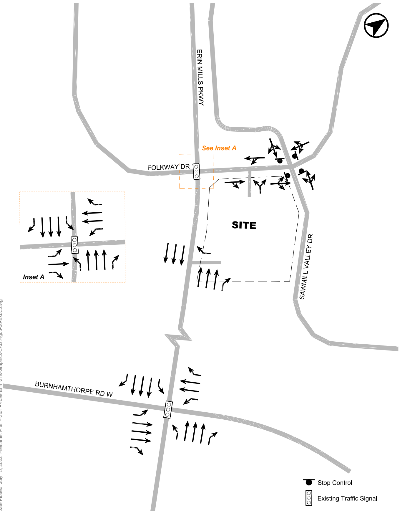
FIGURE 5 EXISTING LANE CONFIGURATION AND TRAFFIC CONTROL
