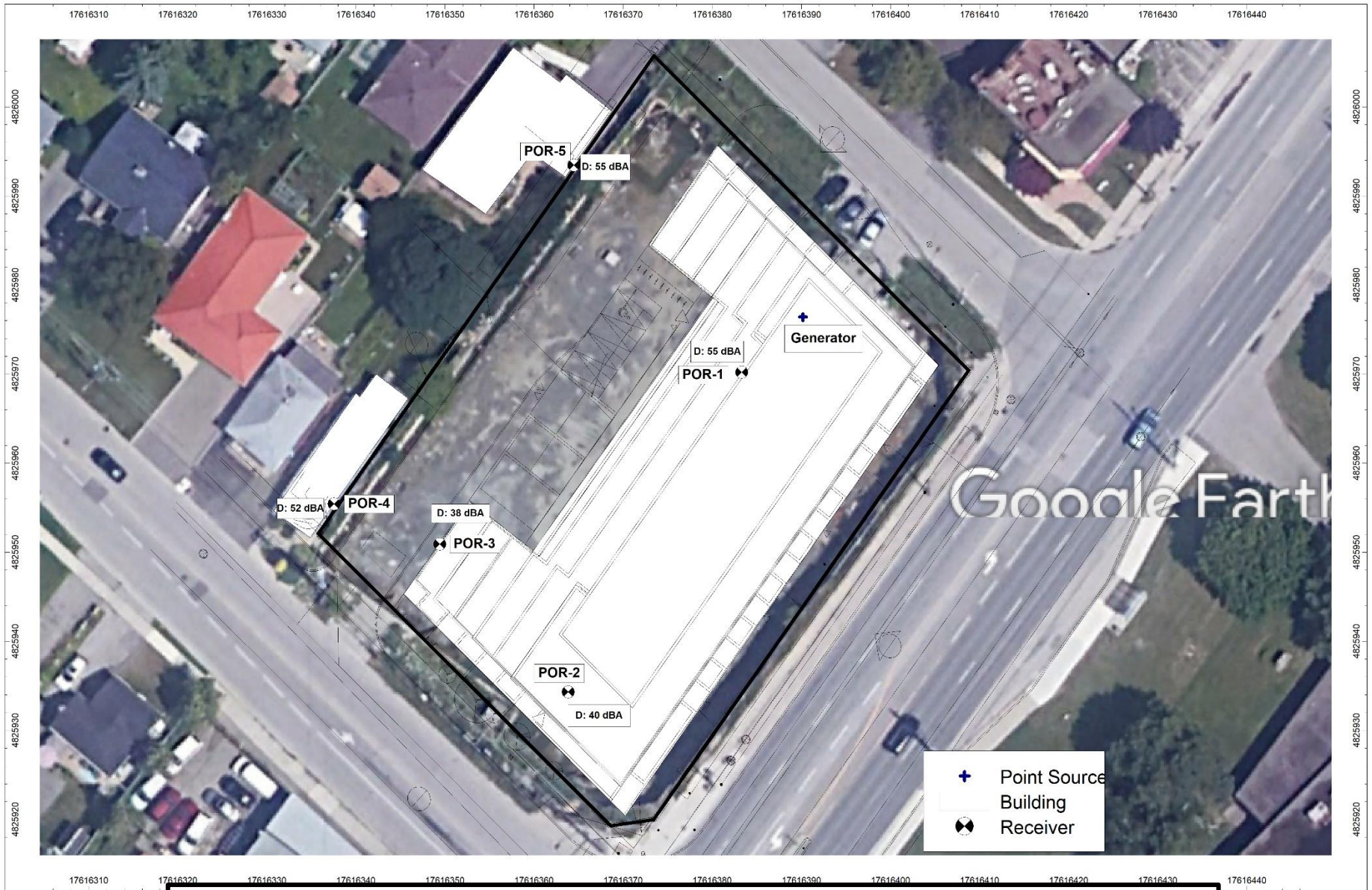
FIGURE 7 IMPACT ASSESSMENT OF EMERGENCY POWER GENERATOR NOISE
