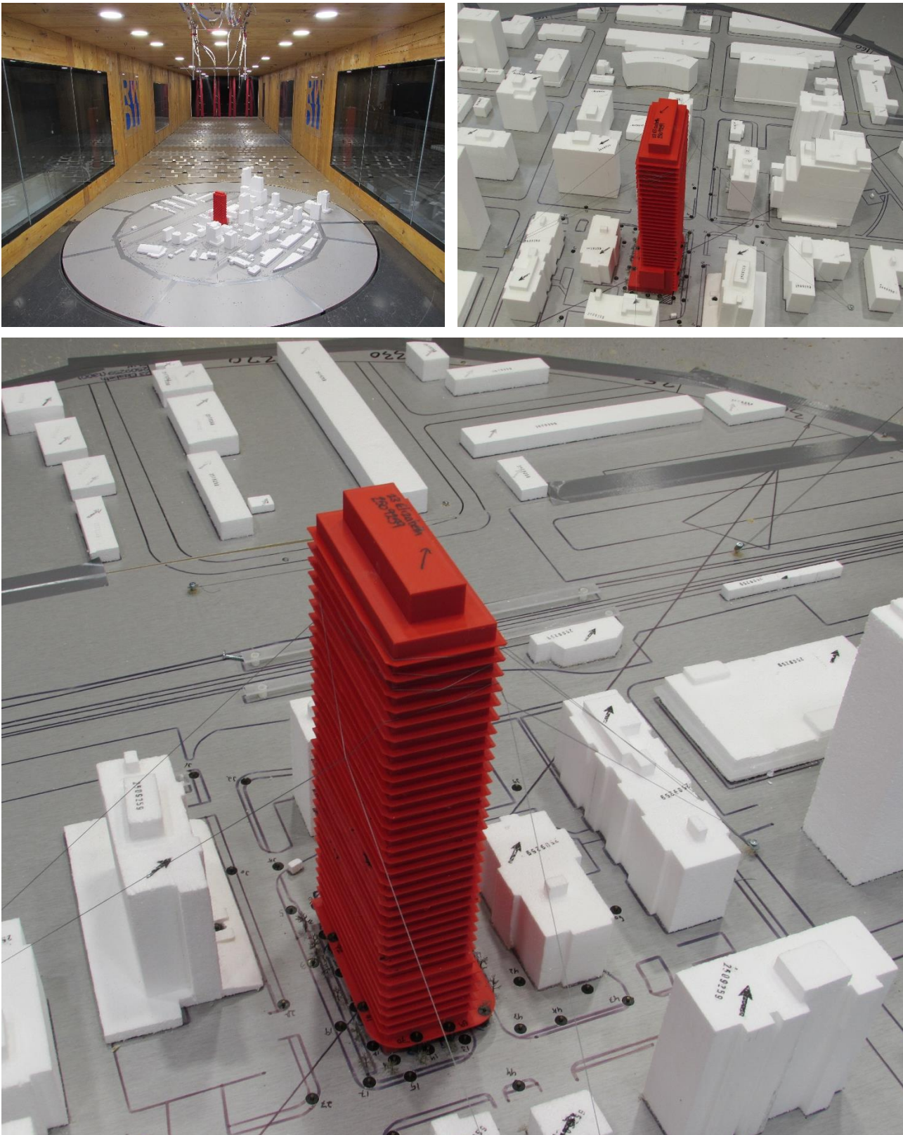
Image 2B: Wind Tunnel Study Model – Proposed Configuration
