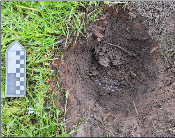
Image 1: Test pit w/ reddish clay on top. Extremely wet and beginning to fill with water. Photo facing north.
