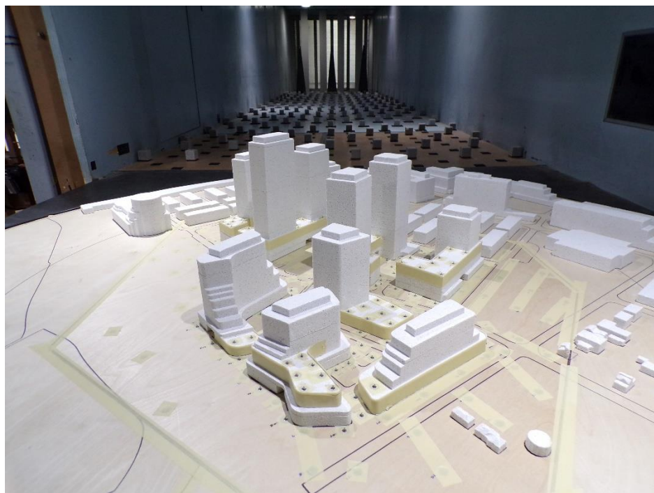
PHOTOGRAPH 2: PROPOSED STUDY MODEL INSIDE THE GWE WIND TUNNEL LOOKING UPWIND
