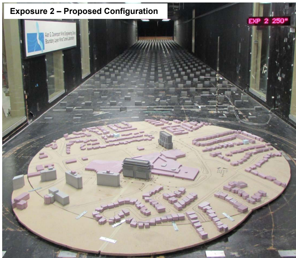
FIGURE 6 PHOTOGRAPH OF THE MODEL IN THE WIND TUNNEL SHOWING THE UPSTREAM TERRAIN MODEL (EXPOSURES) USED
