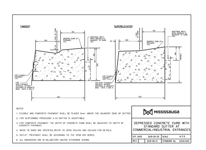
5 DEPRESSED CONCRETE CURB WITH STANDARD GUTTER
