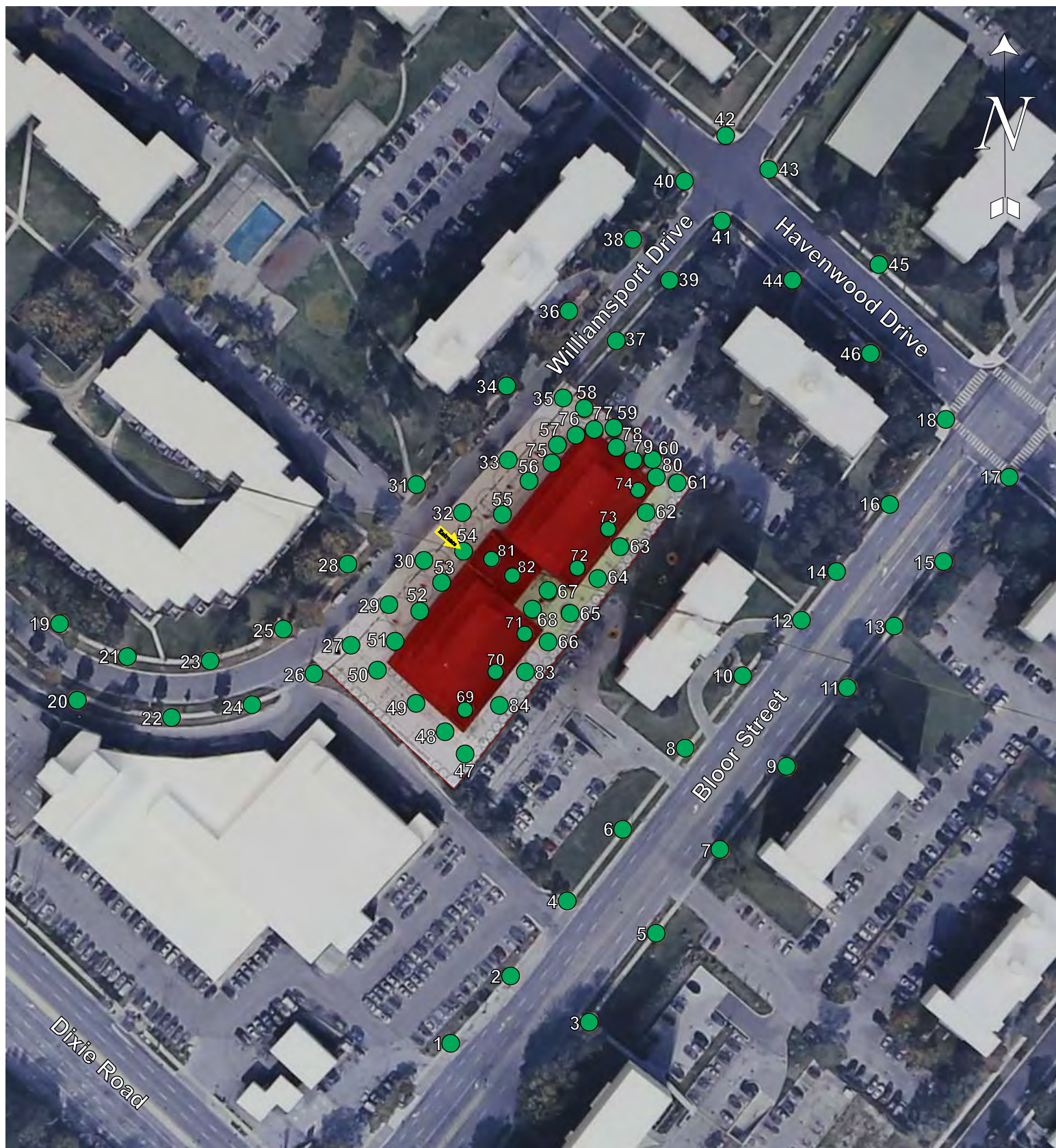
Figure 4: Location plan for pedestrian level wind velocity measurements. 23
