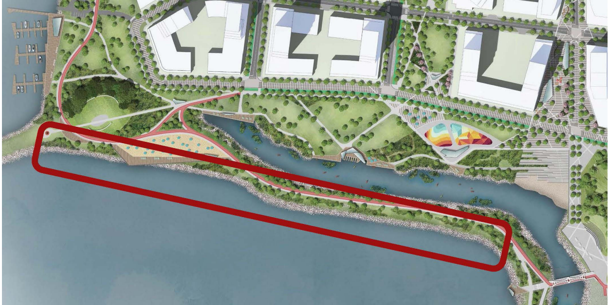
Figure 5.8 - Conceptual plan of the proposed outer shoreline protection repair area, comprising approximately 500 metres of lake facing shoreline edge to meet modern engineering, regulatory flood and erosion protection standards.
