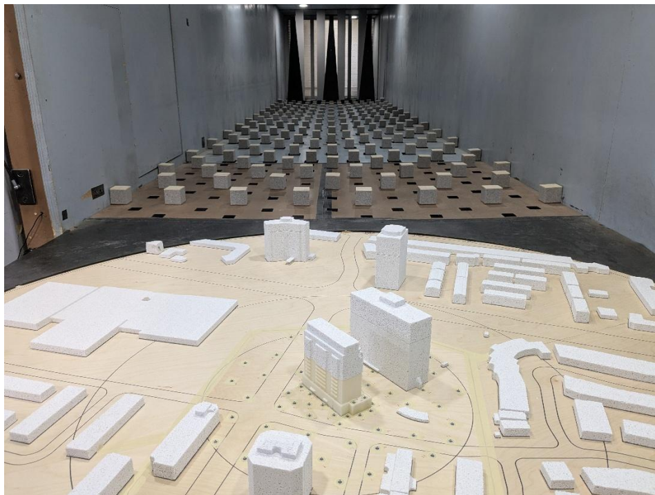
PHOTOGRAPH 4: PROPOSED STUDY MODEL INSIDE THE GWE WIND TUNNEL LOOKING UPWIND
