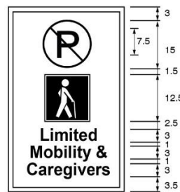
Figure 95: Type-C Parking Signage
