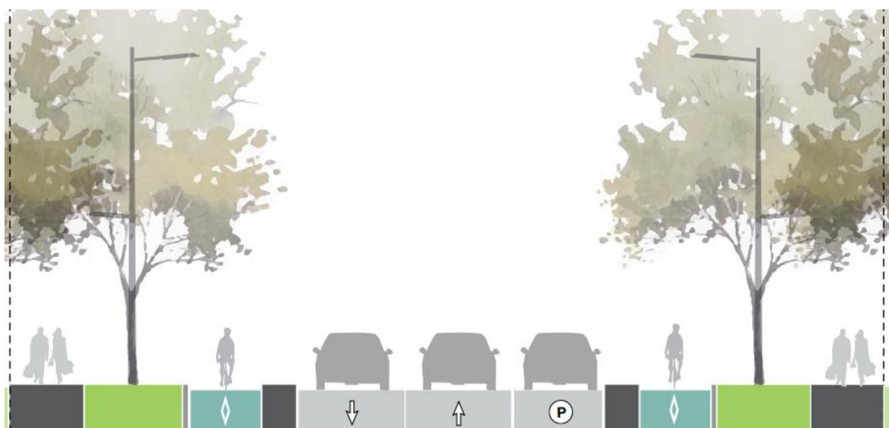
Minor Collector Neighbourhood Typical Section
