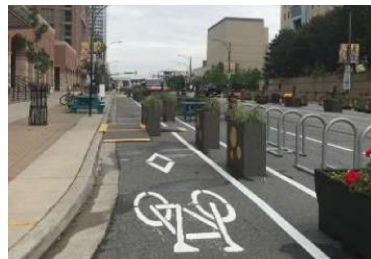
Planters, portable metal bike racks and painted buffer
