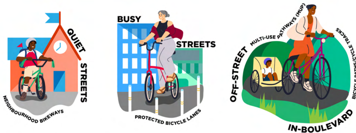
Figure 4.14: To be safe and comfortable for “All Ages and Abilities” (“AAA”) cycling, different facility types are needed depending on the type of roadway.
