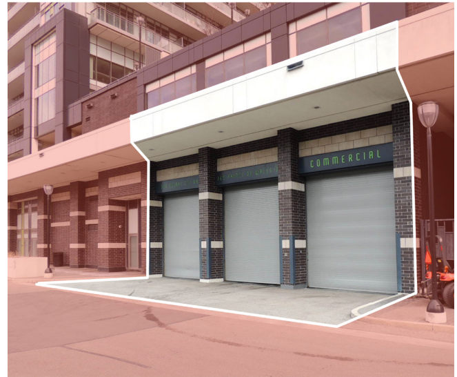
Figure 12: Vehicular access for loading, servicing and parking is designed in a compact fashion and integrated with the building façade.
